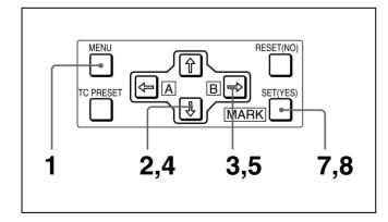
1 Open the door on the lower part of the front panel, then press the MENU button.
